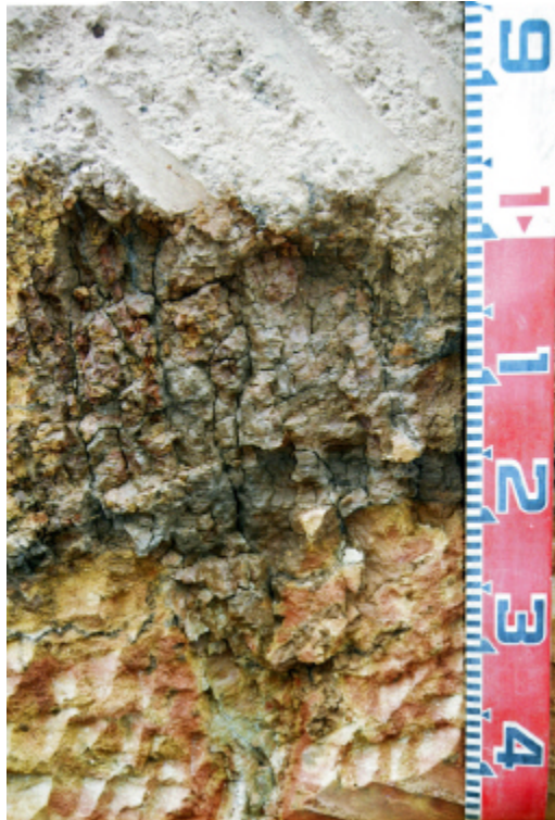
Contrasting soils upslope from SW70 showing deep sandy profile over ferruginised (iron-enriched) sedimentary parent material; profile with thin sodic clay B horizon at 1 metre (left), trench cutting (centre), profile with no clay B horizon and no ironstone gravel (right)
