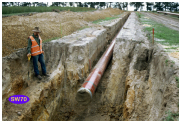
Trench section at site of SW70 showing deep A2 horizon and underlying mottled clay
