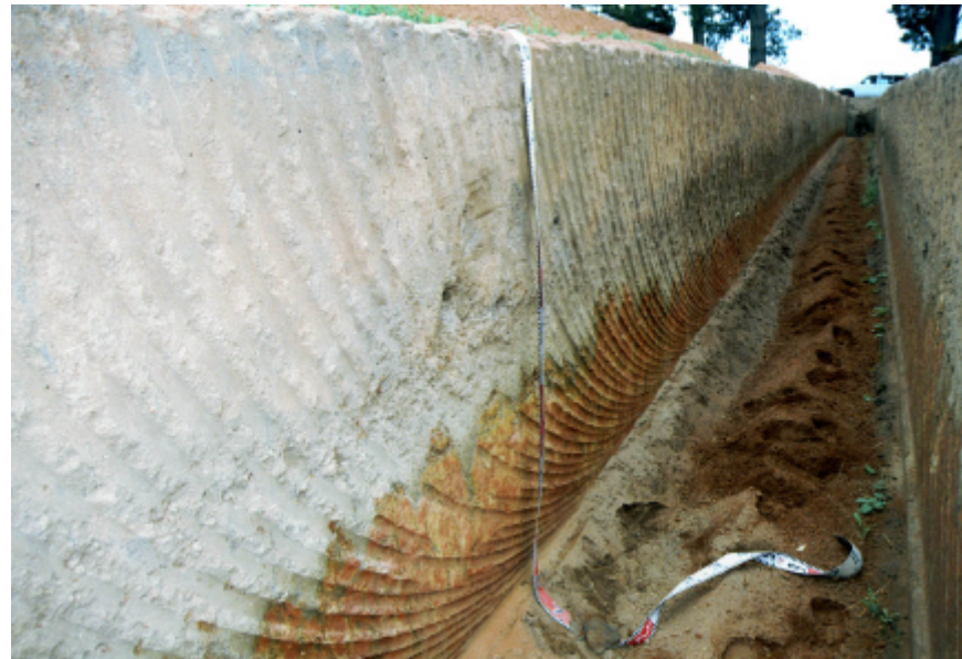
Contrasting soils upslope from SW70 showing deep sandy profile over ferruginised (iron-enriched) sedimentary parent material; profile with thin sodic clay B horizon at 1 metre (left), trench cutting (centre), profile with no clay B horizon and no ironstone gravel (right)
